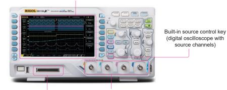
16 digital channels (only available when 4 analog channels DS1000Z Plus has been upgraded)
